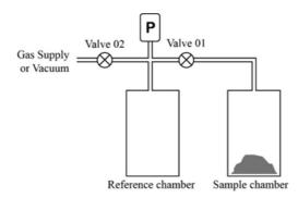
Figure 1: Diagram of Constant Volume Pycnometer
