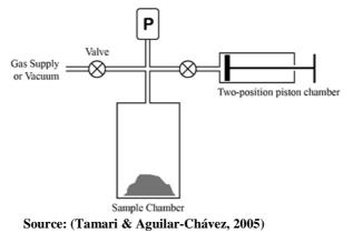
Figure 2: Diagram of Variable-Volume Pycnometer
