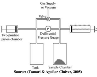
Figure 3: Diagram of a Comparative Pycnometer
